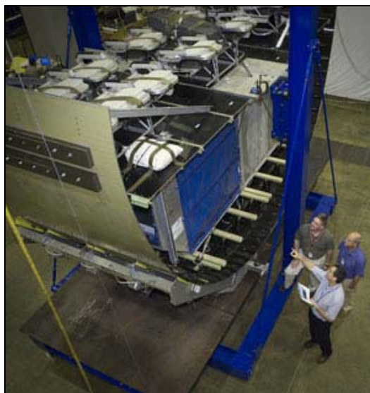
Boeing/Randy's Blog: engineers examine the 787 test rig before the drop test for crash-worthiness.
